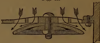
PENN'S DISC VALVE FOR AIR PUMP. Section.
